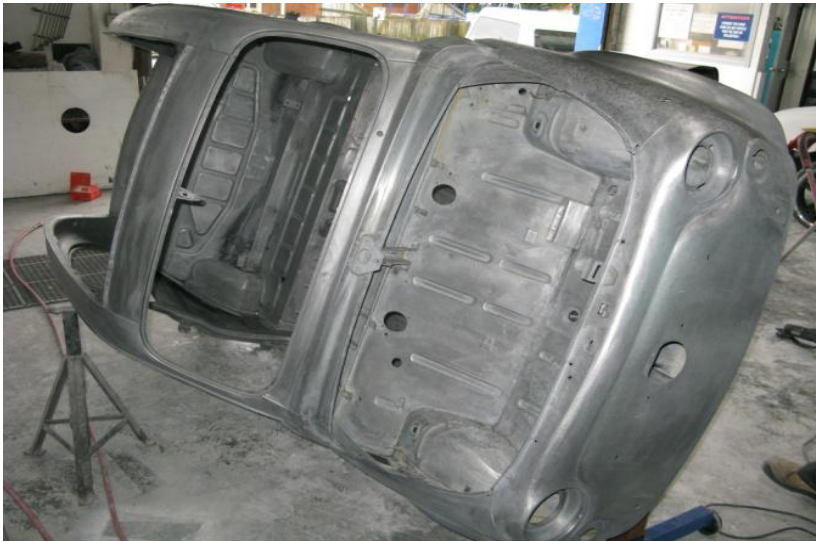
Ready for epoxy.
