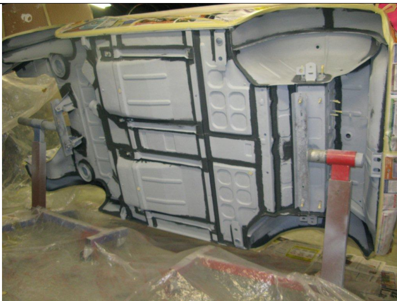
Seamed sealed. Ready for underseal.
